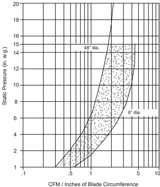
Leakage results shown are based on tests using various damper sizes. The shaded area between the graph lines indicate normal expected leakage range for a standard damper operating conditions and sizes.
